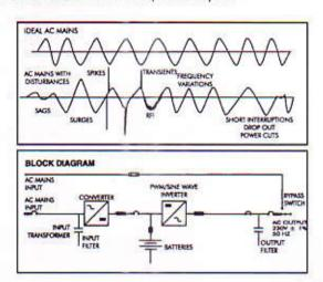
The Static Bypass Switch (optional) available in the UPS System enables transfer of load to the Bypass AC input without interruption in the event of any contingencies. NUMERIC also offers bypass line conditioners such as Isolation Transformers and Servo stabilizers to enhance availability of the UPS System.
